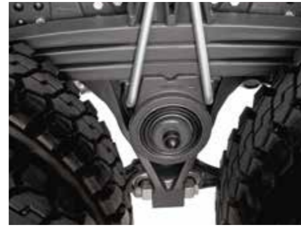
MECHANICAL OR PNEUMATIC REAR SUSPENSION 21 t 3 blade parabolic, 26 t 3 blade parabolic, 21 t 2x2 cushions or 26 t 2x4 cushions.
