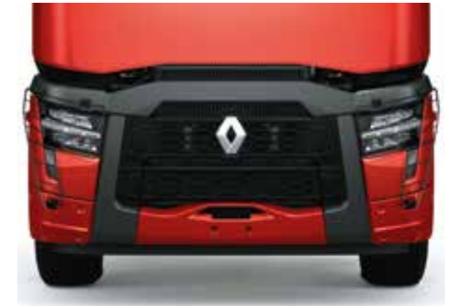
MIXED STEEL / PLASTIC BUMPER with protective grids, for mixed usage (standard).
