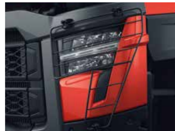
HEADLIGHT PROTECTION GRILLS with standard polycarbonate optics for better impact resistance.
